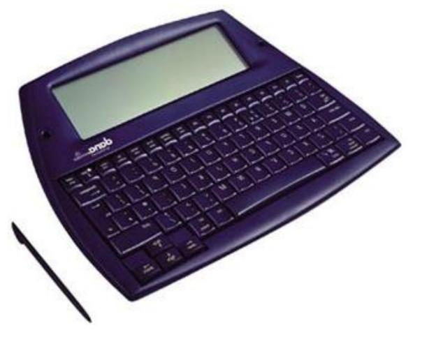
A **portable word processor**, often called a **portable** keyboard, is a lightweight device that is an alternative to using a laptop for writing. It can be easily transported from class to class and between home and school.
